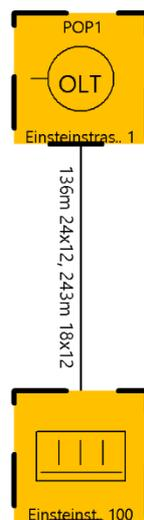
If the cable type to and from the MUC would be the same, the length would be summed up. If the text of a link is too large, you can increase the distance between nodes using the Settings/Distance menu.
